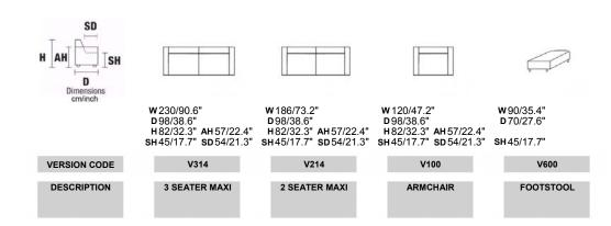
Some versions may be equipped with hidden feet with a supporting structural function.
